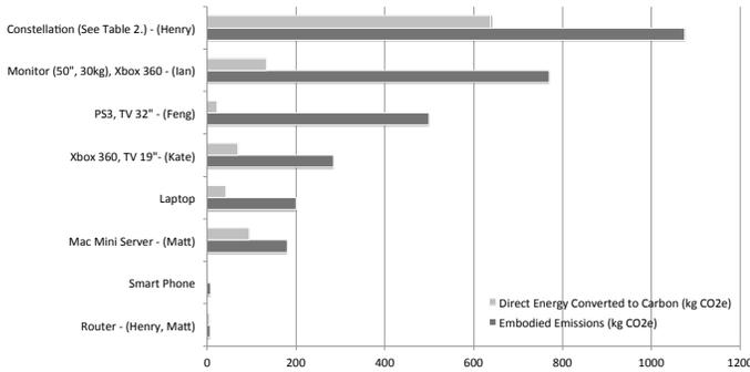
**Figure 2.** Seven examples of the embodied emissions alongside direct emissions. Embodied emissions values are estimated using the values in Table 3. We based our yearly direct emissions estimate on the 20-day energy we observed in the study, and are calculated using the DEFRA 2010 conversion factor, adjusted to include Scope 3 emissions: 0.60 kg CO<sub>2</sub>e/kWh.
